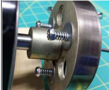
**STEP 11** – Inspect the spanner and magnet spindle to make sure it's held firmly in place. Align the spanner so the threads and washers are centered in hole. It should be tight enough you can move it by hand, but not loose such that it could move from motion of the motor. You may tighten the nuts a little if more pressure is desired, but do not over tighten to avoid bending the aluminum spanner plate.
