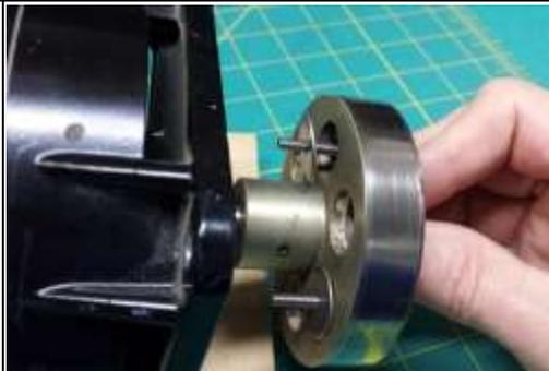
**STEP 8** – Add a spring to each of the threaded studs on the back sides of the washers and finger tighten the lock nuts just enough to hold the assembly in place.
