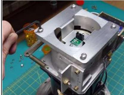
**STEP 16** – Next connect one end of the encoder cable to the encoder and secure the cable to the motor housing with a tie strap. Note the cables are marked TAKEUP and SUPPLY and should be installed on the correct motor for each. The motors are now ready to be installed back into the machine.
