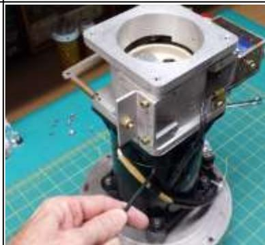
**STEP 14** – Add the magnetic quadrature encoder assembly on the back side of the brake housing.
