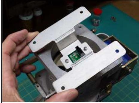
**STEP 15** – Secure the encoder bracket with the lock washers and Allen screws provided. The screws should be tightened snug, but do not over tighten.
