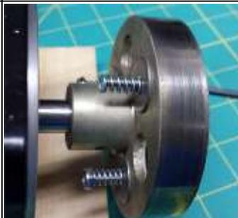
**STEP 9** – Next, tighten the lock nuts with a wrench till the threads just exit the back side of the nylon lock washer. Do not over tighten the screws, the nylon thread locks will hold the screws firmly in place.
