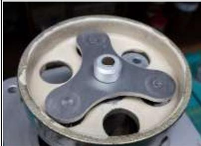
**STEP 7** – Add the large diameter washers on the back side of the brake hub while holding the spindle and spanner in place by hand.
