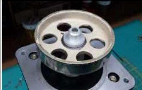
**STEP 5** – Add the spanner bracket over the magnet spindle with the studs and rubber bumpers passing through three of the brake hub cutout holes.
