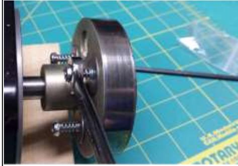
**STEP 10** – The threads should just protrude from the back side of the lock nuts. You may also add some LokTite to the threads if desired. **DO NOT OVER TIGHTEN THE NUTS AND COMPRESS THE SPRINGS TOO TIGHTLY.**
