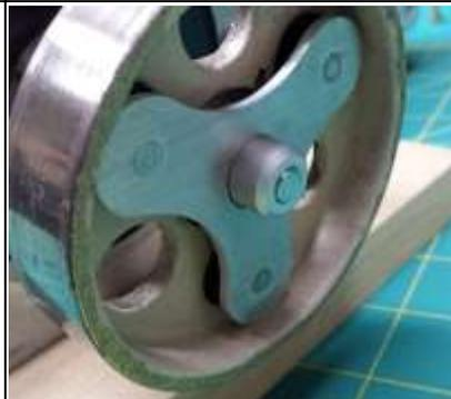
**STEP 12** – Hold the brake solenoid mechanism on the motor to release the brake and spin the motor brake hub by hand. The magnet must spin true without wobble or excessive run out.
