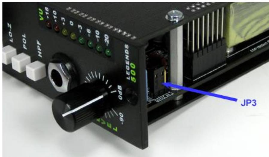
Jumper JP3 allows for three configuration options for the +48V LED on the front panel as shown in the following table.
